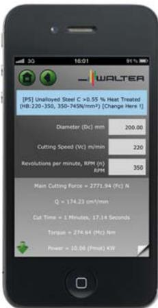
is available for shoulder, face and slot milling, for drilling and counterboring and for ISO turning and grooving. When calculations are made, the material group, rake angle, efficiency factor and wear factor are always taken into account.
